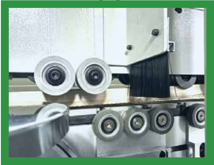
Auxiliary Drag Wheel Prevents damage to the board surface, ensuring stable movement along the conveyor belt and enhancing the stability of the edge banding process.
