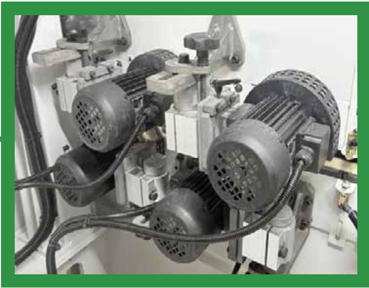
Dual Quick-Release Buffing Units Designed for different colors of board/glue combinations. Ensures the edge banding is glossy and cleaner in appearance.
