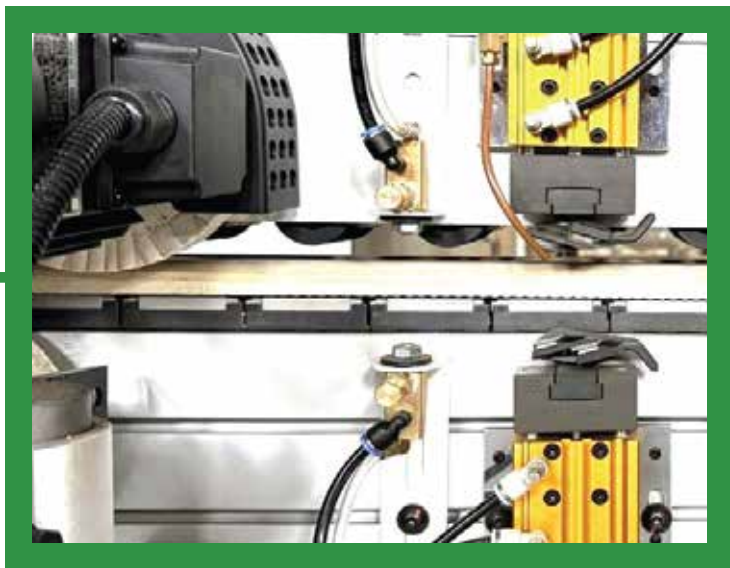
Flexible Flat Scraper + Cleaning Agent Device
