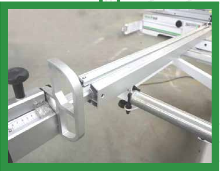
European style parallel fence Stable and accurate. Angle adjustable.
