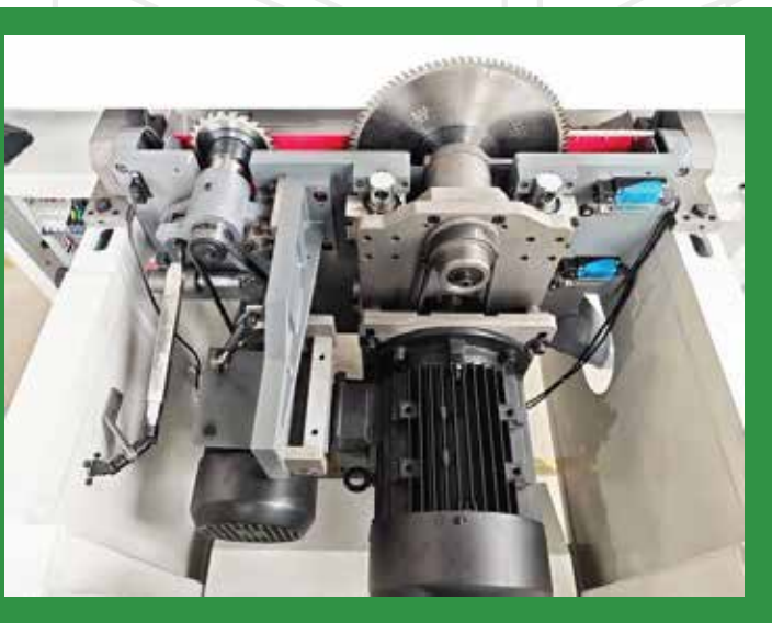
Double saw blade design + high speed motor
