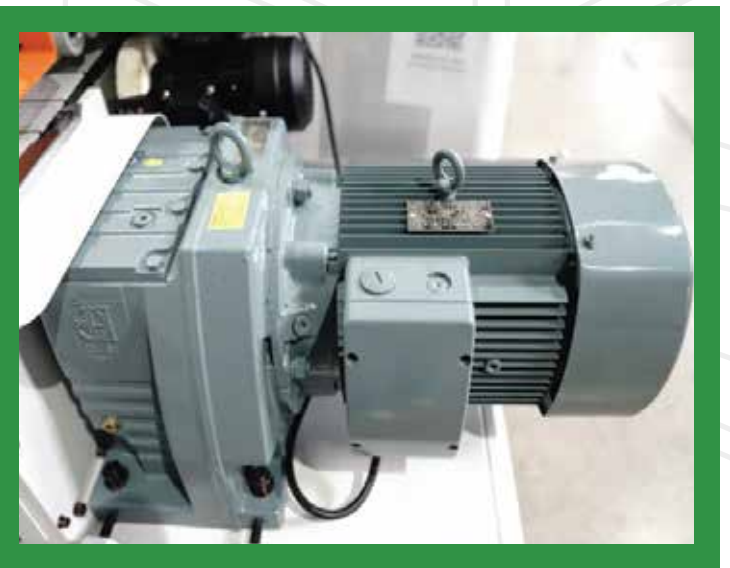
Deceleration motor 4kw power, stable operation.
